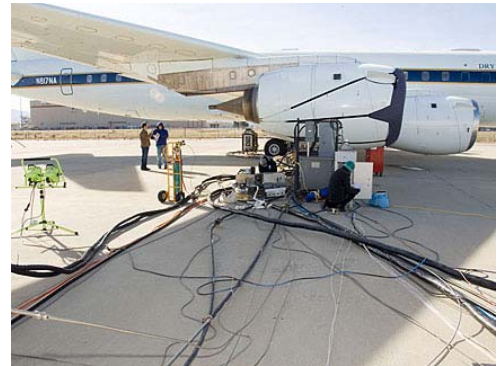
Sampling tubing and instrumentation control cables laid out on the pavement beside NASA's DC-8 flying laboratory in between synthetic fuels emission and engine performance tests at the Dryden Aircraft Operations Facility in Palmdale, Calif. Credit: Tom Tschida, NASA.
